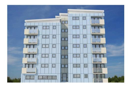
As well as replacing the current external wall insulation with new cladding, we will be replacing all the existing plastic windows and doors with high performance aluminium clad timber windows and doors.
